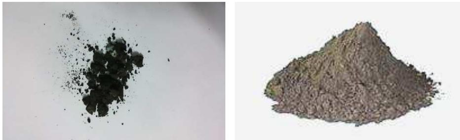
**Figure 1: CuO Nanoparticles (a) Before Sintering (b) After Sintering**
